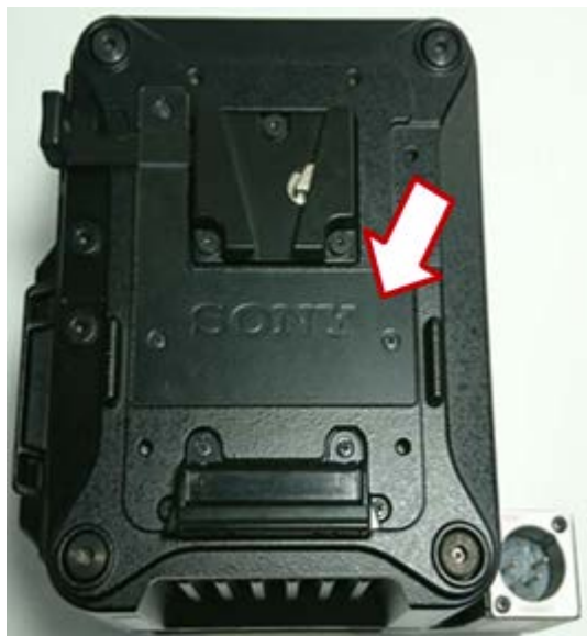
Unscrew the L-Shape Cover (3 Screw)
