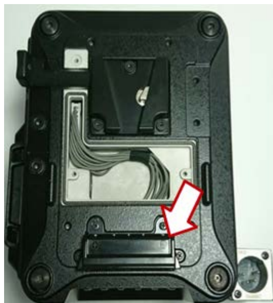
Unscrew the 5Pin connector (4 Screw)
